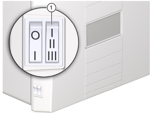
Fig. 21: Reset filter change indicator
