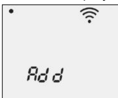
Fig. 10: Connect new ventilation unit
