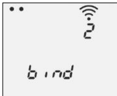
Fig. 14: Connection menu (2 ventilation units already connected)
