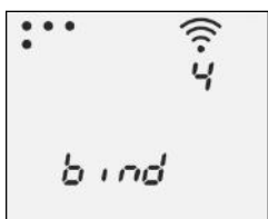
Fig. 9: Connection menu (4 ventilation units already connected)
