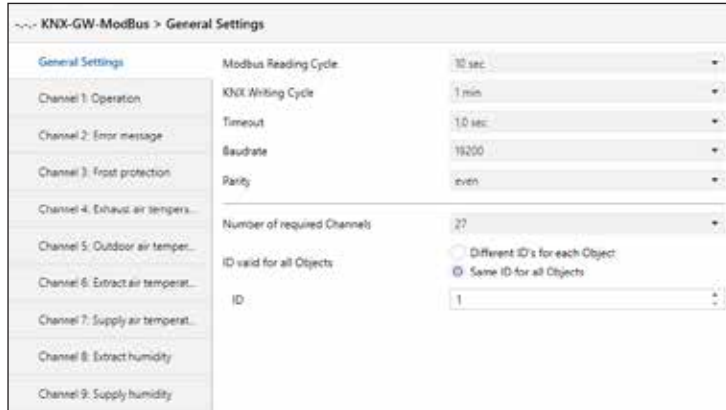
Fig. 6: Factory settings for the KNX gateway
