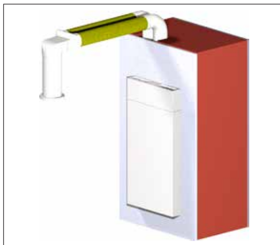
Fig. 4: Flush-mount installation with ductwork connection
