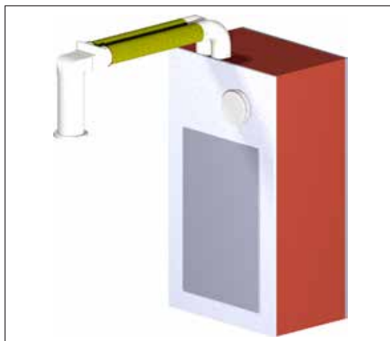
Fig. 5: U 2 integrated into wall installation with ductwork connection
