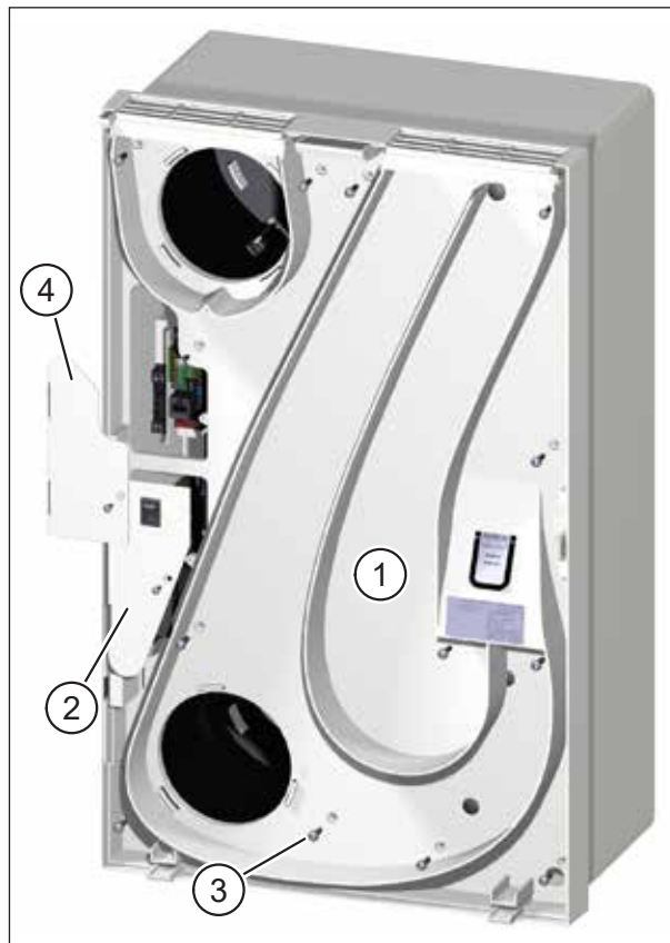
Fig. 26: Insert and secure intermediate plate and electronics compartment covers
