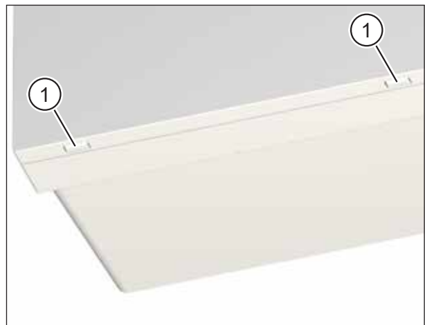
Fig. 22: Removing the cover from the ventilation unit
