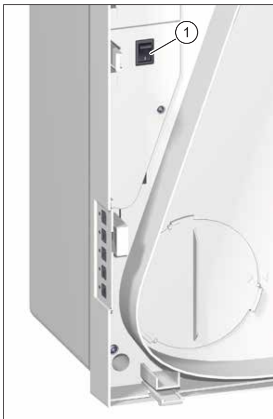
Fig. 13: Mains switch, visible when unit cover is removed
